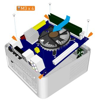
Carefully lower the motherboard into the chassis, with the I/O port side leading so that the ports align with the I/O shield holes and can fit correctly.
